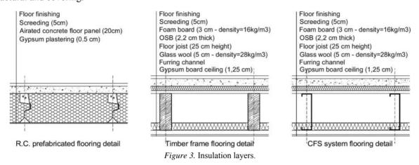
Floor and wall elements are prefered as airated concrete panels in System 1. The reason for using airated concrete panels as a constructional component is to obtain directly over stock. Airated concrete wall panel 20 cm thick exterior wall, 10 cm thick interior wall and airated concrete floor panel 20 cm thick are used in the project (Ayaydın & Koman, 2004; YTONG (aerated concrete manufacturer), 2008).
