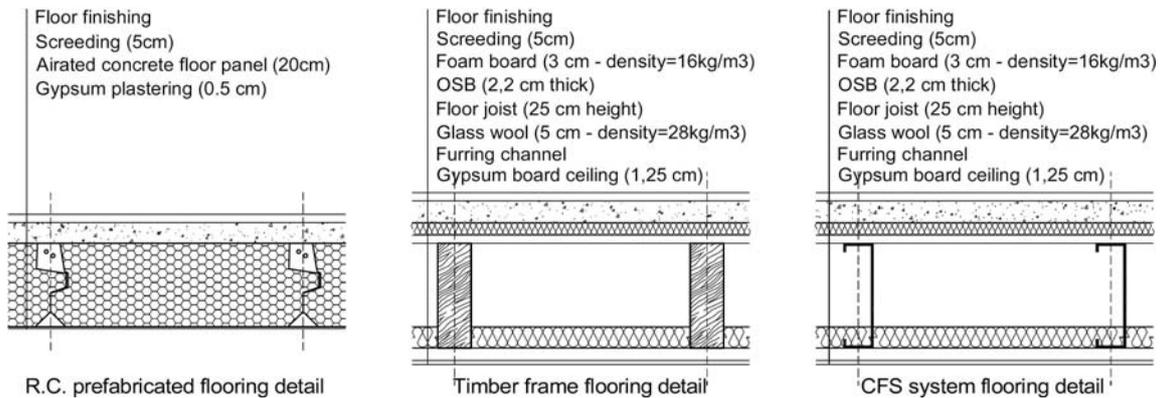
Figure 3. Insulation layers.
