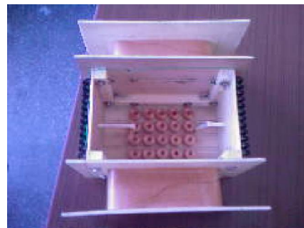
Figure 1. Helmholtz coils and the sensor group
