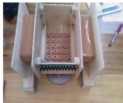
Figure 6. The device measuring the anomaly of a disc-shaped part of a land mine.
