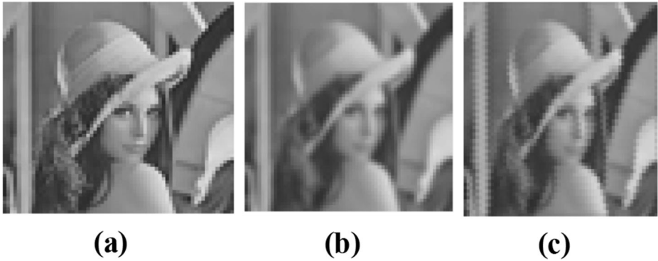
Fig. 14 (a) The original Lena image (b) Lena blurred by the Gaussian kernel on the square domain (c) Lena blurred by the Gaussian kernel on the hexagonal domain
